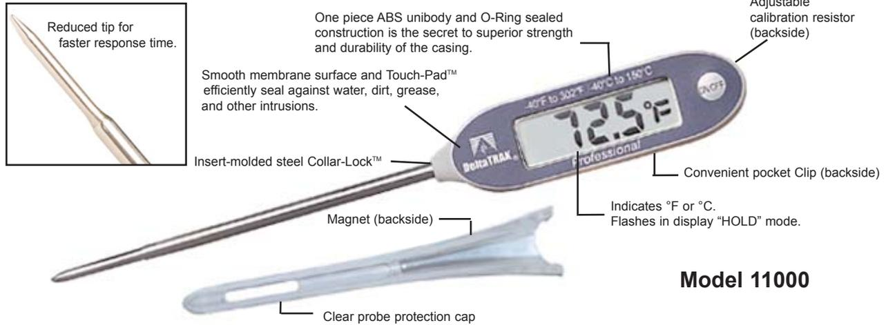
This unique, next-generation, digital pocket probe thermometer is engineered to set the industry standard for accuracy, durability and readability. It is designed and constructed under exacting standards to meet and exceed the specifications required for commercial and industrial uses.
